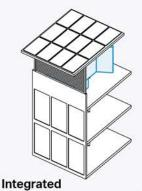
Curved ParapetIThe parapet begins to curve intoIthe Hover wind turbine unit,Iproviding more efficient air flow.I
