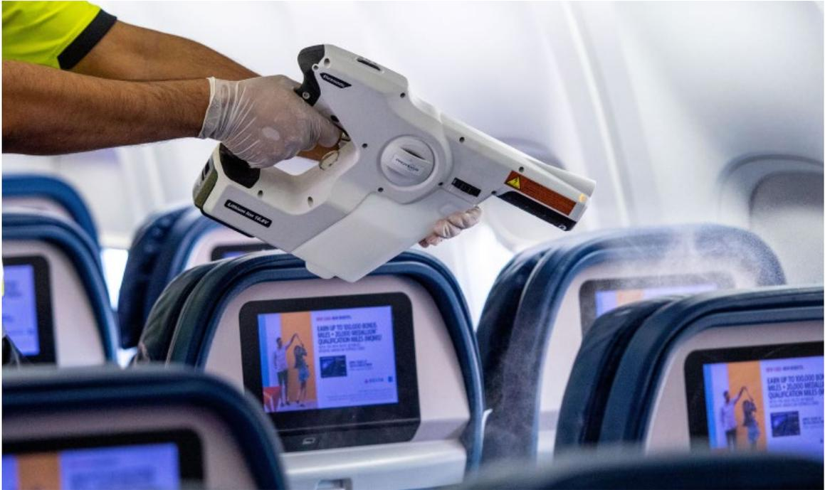
Figure 1: Electrostatic Fogging; Photo Courtesy of Delta Air Lines
